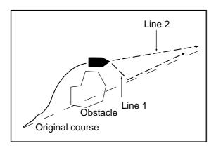
Figure 8-7 Example of when to restart navigation
